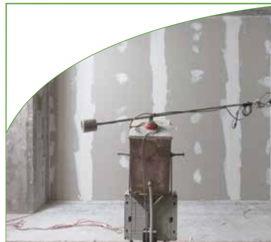
Airborne sound laboratory test Trocellen false wall
