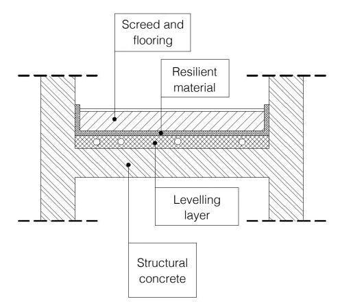
If correctly positioned, the springy sound-proofing acts like a spring to dampen any drum sound vibration caused by people walking on the floor. It is therefore essential that the following instructions are observed.
