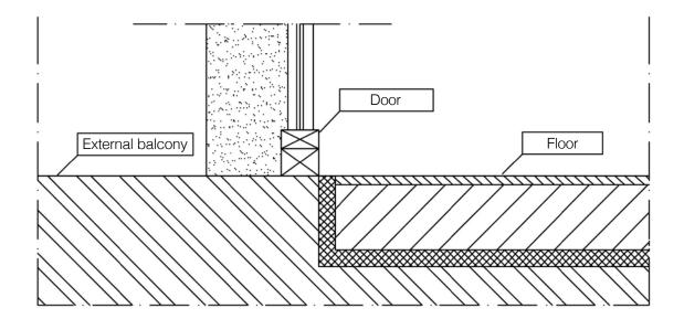
Both the skirting-boards and the wall-tiles in bathrooms and kitchens must be a few millimeters apart from the flooring to avoid the formation of rigid connections between the floor and the walls.
