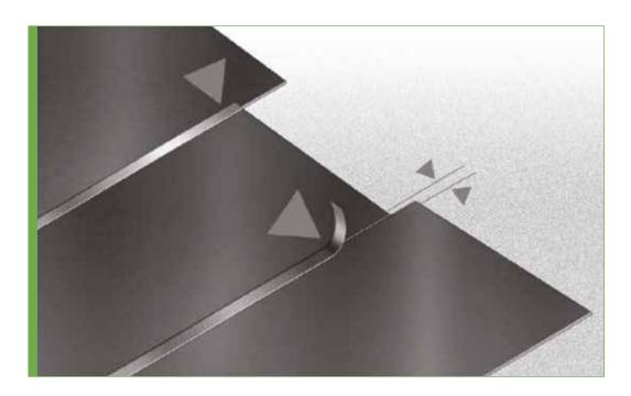
If the springy sound-proofing is fibrous or porous (e.g. panels of fiber-glass panels or high density rock-wool, high density polyester panels, etc.) or has a fibrous or porous surface layer (e.g. a crosslinked poly-ethylene foam/polyester laminate), it must not be allowed to soak up the concrete during casting. Therefore, protect the sound-proofing before casting by covering it with overlapping sheets of poly-ethylene taped together.
