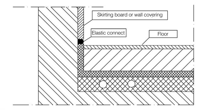
In the event a floor heating system is installed, make certain that the floating floor and the external structures is not connected. Therefore to ensure that vibrations are not transmitted, make certain to:
