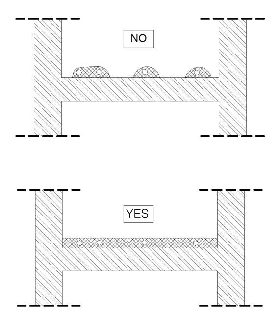
If the cables and pipes are covered with lightweight material, check that this is of the same quality and density across the floor.
