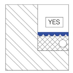
We recommend reinforcing the concrete with a net. You should also take into account the type of the resilient material used.
